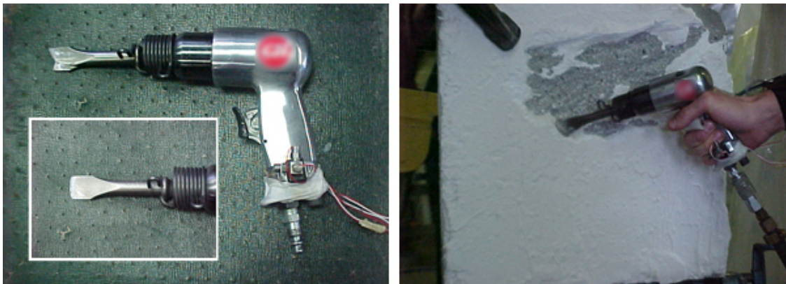
Figure 3.3: (a) Impact Hammer Instrumented with Tri-axial Accelerometer and Fitted with Flat Chisel and Splitter Bits and (b) Impact Hammer In Use
