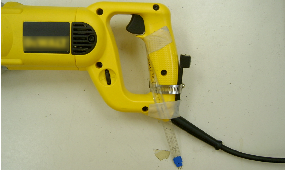
Figure 3.6: Reciprocating Saw Instrumented with Finger Pressure Sensor
