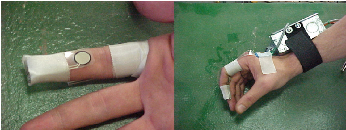
Figure 2.3: DC Electronic Finger Pressure Instrumentation System – Pressure Sensor and Preamplifier
