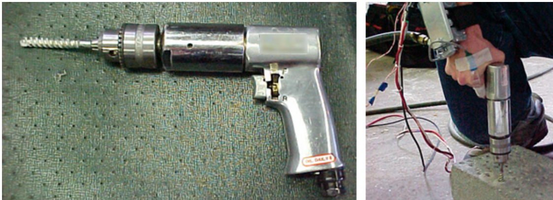
Figure 3.4: (a) Pneumatic Drill with 3/8" Masonry Bit and (b) Drill In Use
